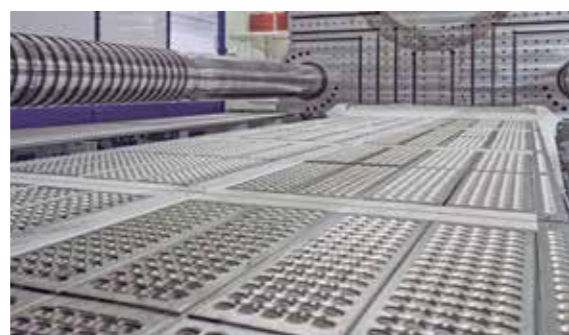
Equipped with a large-area safety pedal to provide safety protection for the mold clamping area (9000kN and above).
